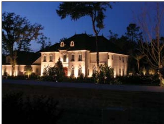
The front façade is brightly lit with 35-watt uplights that are softened and dispersed with frosted lenses. The open area between the approach and the home highlights the stark contrast.
