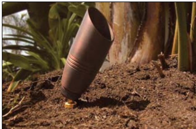
This MR16 halogen bullet light is placed directly into the ground with a seven-inch brass stake attached to the unit. Close to 100 stake-mounted bullet lamps were used on the project with 11 transformers and one synchronized master controller.
